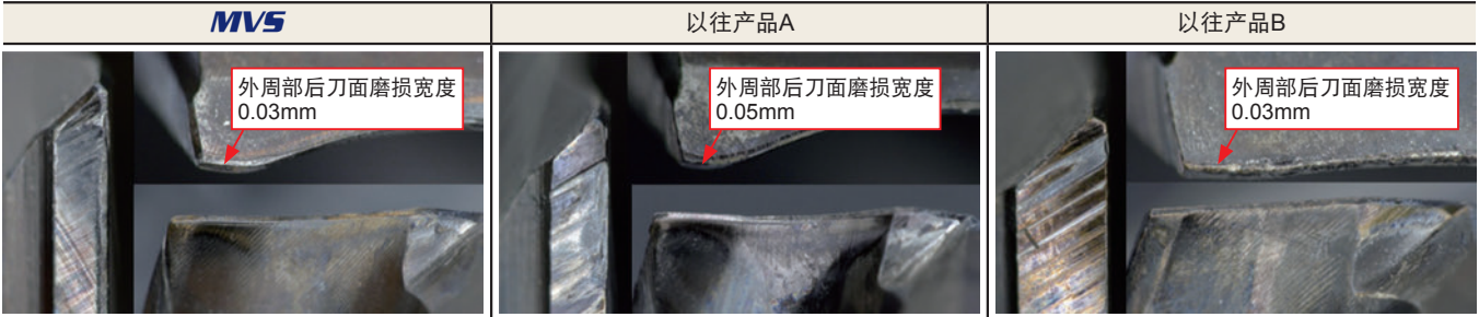
切削长度55m时的刀尖损伤状态
